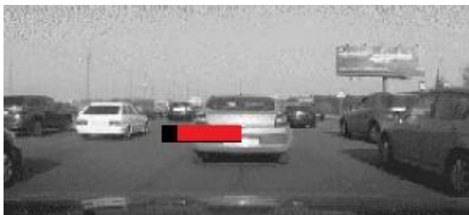
Figure 5 – On-chip analytics is a particularly effective way of spotting anomalous states in sensors, such as stuck pixels within a camera system. This can be achieved non-intrusively and at system speed, providing early warning of fault conditions before they manifest as operational failures
