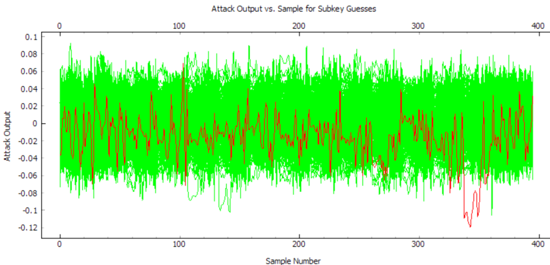
Figure 4: Attack output vs sample number for subkey guesses. The leakage that lets an attacker deduce each key byte is frequently isolated to specific groups of calculations and is often identified by changes in correlation. In this example, a large change in correlation in the region around 350 samples shows the results of a correctly guessed key byte.
