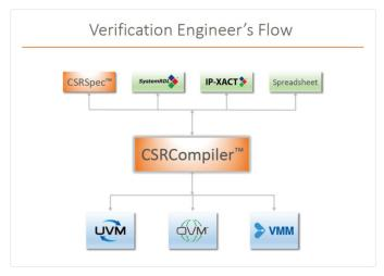
CSRCompiler accepts IP-XACT, SystemRDL, spreadsheets and CSRSpec to generate both industry standard output and output customized for design teams.
